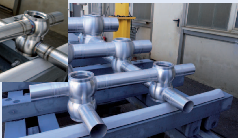
Stainless steel surface before (above) and after (right) Rotainer® pickling
